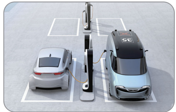
Charging station for bus and taxi and highway rest stop Equipment: High-power AC and DC chargers Feature: Low density, rapidity, safety
